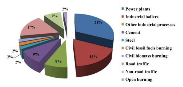
Fig. 2-1 China's NO<sub>x</sub> emissions sources and distribution in 2010
