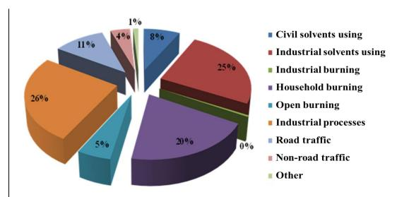
Fig. 2-2 China's VOCs emissions sources and distribution in 2010
