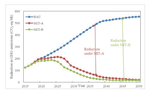
Fig. 3-2 HFCs emission reduction potential for room air conditioners in China, 2016-2050
