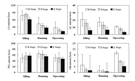
(b) Fuel-based emission factor of agricultural machinery (g/kg fuel consumption)
