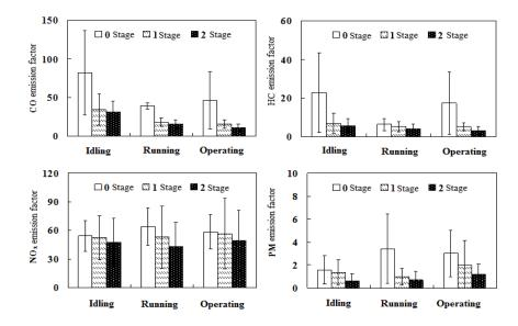
(a) Fuel-based emission factor of construction machinery (g/kg fuel consumption)
