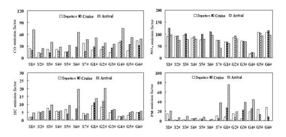
(c) Fuel-based emission factor of inland vessels (g/kg fuel consumption)
